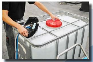
Open the IBC-screw-lid and put the special splash-guard-lid on the IBC-opening.
