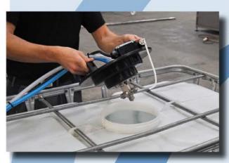
A conical splash guard lid ensures an optimum hold and is adapted to the standardized openings of IBC's.
